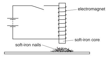
The switch is now closed, left closed for a few seconds, and then opened.
