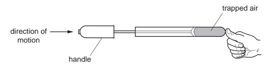
What happens to the pressure and what happens to the volume of the trapped air as the pump handle is pushed in?
