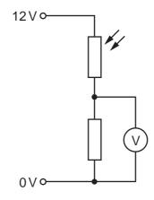
The light falling on the light-dependent resistor (LDR) increases in brightness.
