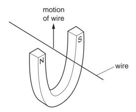
Which device uses a moving wire to induce an e.m.f.?
