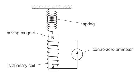
What does the ammeter show when the magnet repeatedly moves slowly up and down?
