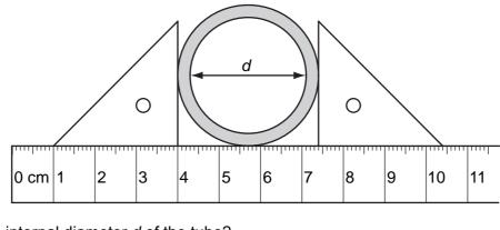
What is the internal diameter d of the tube?
