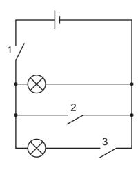
Which switches must he close to light both lamps?
