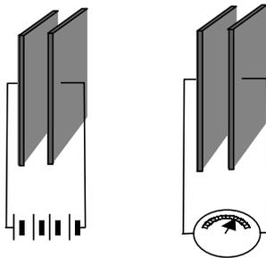
The capacitor is first connected to a d.c. supply and then to a sensitive ammeter (or galvanometer). When the capacitor is connected to the sensitive ammeter, a *momentary* deflection is observed. This deflection is a brief pulse of *charge* and illustrates an important idea with capacitors.
