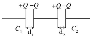
You can see this by looking at the two inner plates, one from each capacitor, and remembering that they are insulated from the rest of the circuit. The charge lost by one plate must equal that gained by the other. The total charge stored here is  $Q$ .
