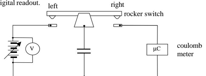
By depressing the left hand key of the rocker switch, the capacitor is charged to a potential difference  $V$  which can be adjusted by the variable d.c. supply. Upon depressing the right hand key, the stored charge  $Q$  is measured and displayed by the coulombmeter.
