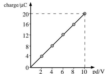
The ratio  $\frac{Q}{V}$  is the gradient of the straight line, so  $\frac{Q}{V} = \text{constant}$
