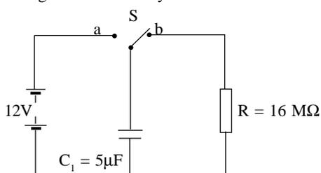
Calculate the charge on  $C_1$  60 seconds after closing S.
