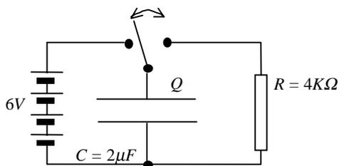
The answer is displayed in graph below. It shows the charge Q remaining on the capacitor. The initial charge is found by using  $Q = CV$ :  $Q_0 = 2\mu \times 6 = 12\mu C$  as shown on the graph.
