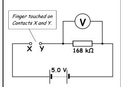
(b) When the finger makes contact between X and Y, the voltmeter reading changes from O V to 3.4 V because of the electrical resistance of the skin. Use this information to calculate the electrical resistance of the skin between the two contacts.
