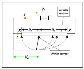
By moving the sliding contact on the variable resistor, the value of the OUTPUT PD ( $V_o$ ) can be adjusted:
