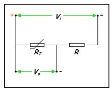
The resistance of a positive temperature coefficient (PTC) thermistor increases.
