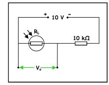
(b) The value of  $R_L$  in lighting conditions for which  $V_o = 4.0 \ V$ .
