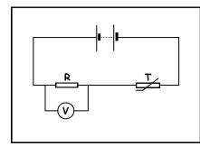
**Describe** and **explain** how the voltmeter reading changes as the temperature of the greenhouse **increases**.
