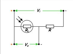
An LDR is a resistor made from semiconducting material in which electrons are liberated when light shines on the surface of the material.
