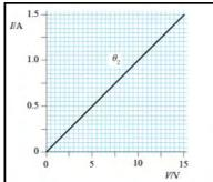
The above graphs show the I-V characteristics for a metal wire at two different temperatures  $\theta_1$  and  $\theta_2.$
