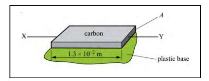
The **resistance** of the carbon layer between X and Y is = 2200  $\Omega$ . The **length** of the carbon layer is =  $1.3 \times 10^{-2}$  m. The **resistivity** of carbon is =  $3.5 \times 10^{-5} \Omega$ m.
