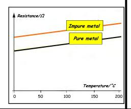
The <u>RESISTANCE</u> of an <u>IMPURE</u> metal also <u>increases</u> <u>linearly with increasing</u> temperature, but it is <u>greater</u> than that of a PURE metal.
