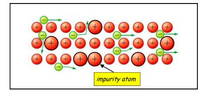
The fact that the impurity atoms and the metal ions are different in size causes an increase in the frequency of the collisions experienced by the drifting electrons. This extra opposition to the flow of electrons means that the resistance is made greater by the presence of impurity atoms in the metal.
