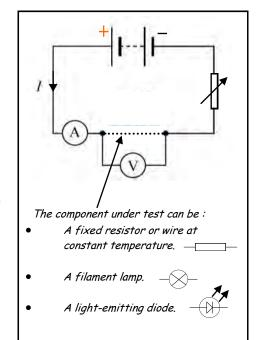
Alternatively, an ammeter sensor and a voltmeter sensor connected to a data logger can be used to measure and record corresponding I-V readings which can then be displayed directly on a computer screen.
