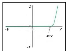
For pd (V)  $\langle \approx 2V$ , the current (I) is  $\approx 0$ , so the LED has almost infinite resistance. The LED starts to conduct at its threshold pd ( $\approx 2V$ ) and its resistance decreases dramatically for pd's > 2V.
