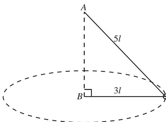
A light inextensible string of length  $8l$  has its ends fixed to two points  $A$  and  $B$ , where  $A$  is vertically above  $B$ . A small smooth ring of mass  $m$  is threaded on the string. The ring is moving with constant speed in a horizontal circle with centre  $B$  and radius  $3l$ , as shown in the diagram above. Find
