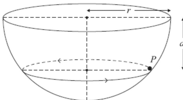
A particle  $P$  of mass  $m$  moves on the smooth inner surface of a hemispherical bowl of radius  $r$ . The bowl is fixed with its rim horizontal as shown in the diagram above. The particle moves with constant angular speed  $\sqrt{\left(\frac{3g}{2r}\right)}$  in a horizontal circle at depth  $d$  below the centre of the bowl.
