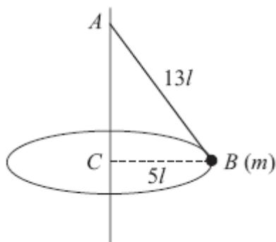
A garden game is played with a small ball  $B$  of mass  $m$  attached to one end of a light inextensible string of length  $13l$ . The other end of the string is fixed to a point  $A$  on a vertical pole as shown in the diagram above. The ball is hit and moves with constant speed in a horizontal circle of radius  $5l$  and centre  $C$ , where  $C$  is vertically below  $A$ . Modelling the ball as a particle, find
