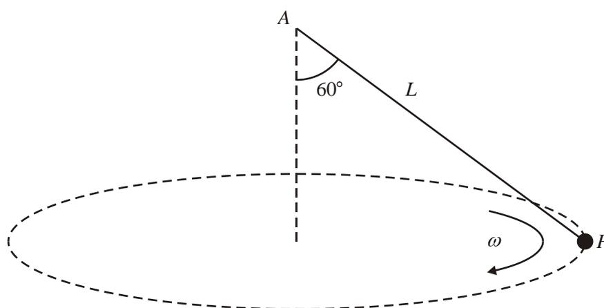
A particle  $P$  of mass  $m$  is attached to one end of a light string. The other end of the string is attached to a fixed point  $A$ . The particle moves in a horizontal circle with constant angular speed  $\omega$  and with the string inclined at an angle of  $60^\circ$  to the vertical, as shown in the diagram above. The length of the string is  $L$ .
