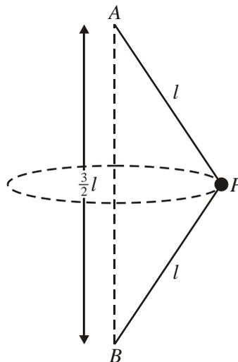
A particle  $P$  of mass  $m$  is attached to the ends of two light inextensible strings  $AP$  and  $BP$  each of length  $l$ . The ends  $A$  and  $B$  are attached to fixed points, with  $A$  vertically above  $B$  and  $AB = \frac{3}{2}l$ , as shown in the diagram above. The particle  $P$  moves in a horizontal circle with constant angular speed  $\omega$ . The centre of the circle is the mid-point of  $AB$  and both strings remain taut.
