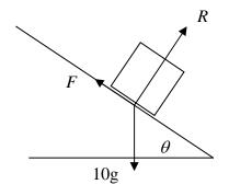
Resolving perpendicular to the slope:  $R = 12g \cos \theta$ Resolving parallel to the slope:  $F = \mu R = 12g \sin \theta$   $\therefore \quad 0.6 \times 12g \cos \theta = 12g \sin \theta$   $\tan \theta = 0.6$   $\theta = 31^{\circ}$ i.e. the block will slide at an angle of 31
