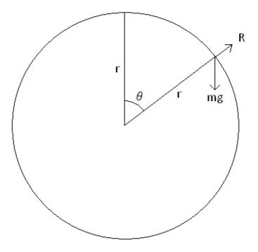
For the ball-bearing to leave the sphere, the normal reaction must reach 0.
