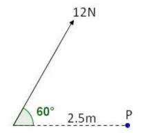
The moment of the 12*N* force acting on point *P* has a magnitude equal to:
