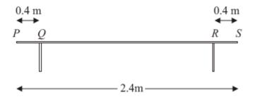
A bench consists of a plank which is resting in a horizontal position on two thin vertical legs. The plank is modelled as a uniform rod PS of length 2.4 m and mass 20 kg. The legs at Q and R are 0.4 m from each end of the plank, as shown in the diagram above.
