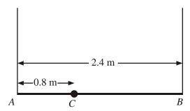
A plank AB has mass 12 kg and length 2.4 m. A load of mass 8 kg is attached to the plank at the point C, where AC = 0.8 m. The loaded plank is held in equilibrium, with AB horizontal, by two vertical ropes, one attached at A and the other attached at B, as shown in the diagram above. The plank is modelled as a uniform rod, the load as a particle and the ropes as light inextensible strings.
