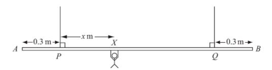
A beam AB is supported by two vertical ropes, which are attached to the beam at points P and Q, where AP = 0.3 m and BQ = 0.3 m. The beam is modelled as a uniform rod, of length 2 m and mass 20 kg. The ropes are modelled as light inextensible strings. A gymnast of mass 50 kg hangs on the beam between P and Q. The gymnast is modelled as a particle attached to the beam at the point X, where PX = x m, 0 < x < 1.4 as shown in the diagram above. The beam rests in equilibrium in a horizontal position.
