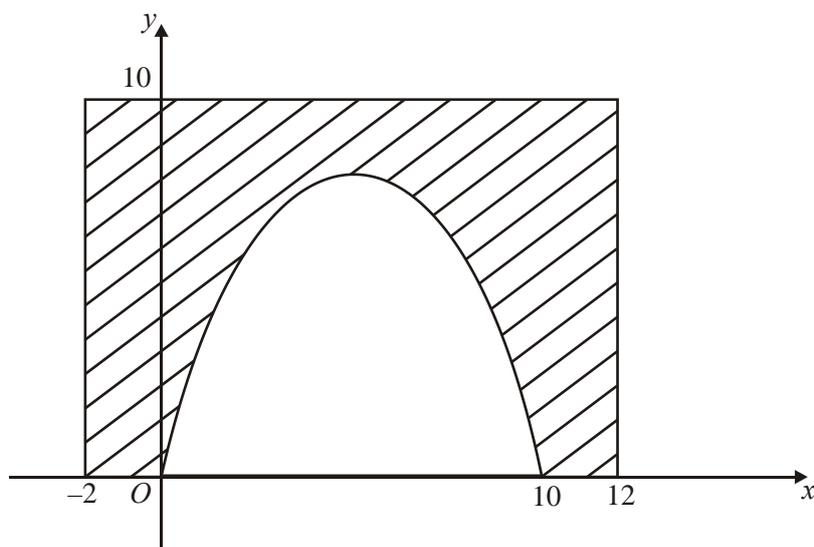
The diagram above shows the cross-section of a road tunnel and its concrete surround. The curved section of the tunnel is modelled by the curve with equation  $y = 8\sqrt{\left(\sin \frac{\pi x}{10}\right)}$ , in the interval  $0 \leq x \leq 10$ . The concrete surround is represented by the shaded area bounded by the curve, the  $x$ -axis and the lines  $x = -2$ ,  $x = 12$  and  $y = 10$ . The units on both axes are metres.
