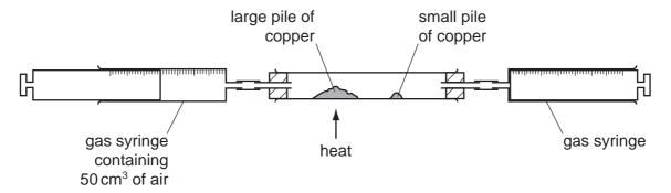
The gas syringe contains 50 cm³ of air. The large pile of copper is heated and the air is passed from one gas syringe to the other over the hot copper. The large pile of copper turns black. The gas is allowed to cool and its volume measured.
