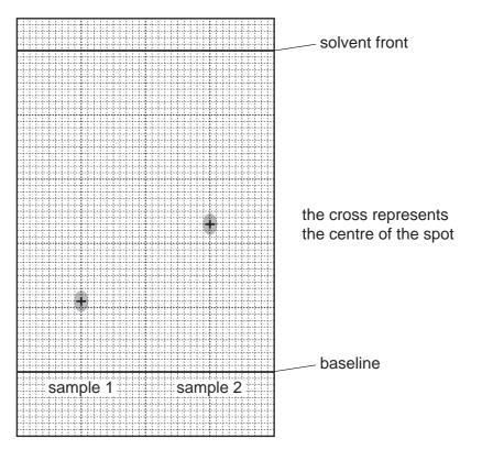
An ester was used as the solvent and the chromatogram was sprayed with bromothymol blue.
