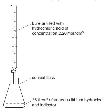
25.0 cm³ of aqueous lithium hydroxide is pipetted into the conical flask. A few drops of an indicator are added. Dilute hydrochloric acid is added slowly to the alkali until the indicator just changes colour. The volume of acid needed to neutralise the lithium hydroxide is noted.
