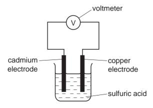
Results from cells using the metals tin, cadmium, zinc and copper are given in the table below.
