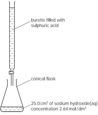
(a) 25.0 cm<sup>3</sup> of aqueous sodium hydroxide is pipetted into a conical flask.
